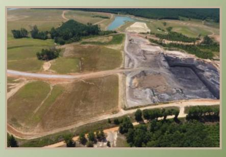
183 acres with 32 acres currently in operation with active mining and reclamation projects. The remaining open acreage includes sedimentation control ponds and overburden stockpiles. The mine supplies approximately 220,000 tons of lignite feedstock annually to AES' carbon activation facility near Coushatta in Red River Parish.
